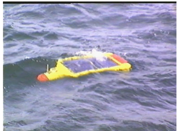
Figure 1. Solar Powered AUV (SAUV)
