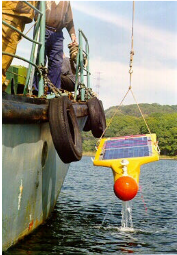
Figure 4. SAUV Vehicle Recovered From Sea Tests
