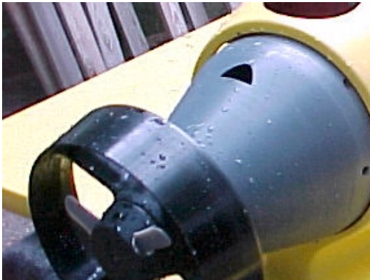
Figure 7. SAUV II Vectored Thruster w/3 Bladed Propeller
